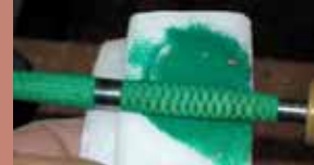
Fig. 5. Set up the mandrel and bushings just as you would with any other material.
